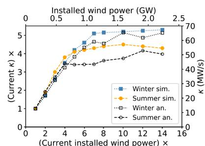
Fig. 2. Secondary control gain parameter  $\kappa$  needed to keep fluctuations within statutory limits as wind capacity increases.
