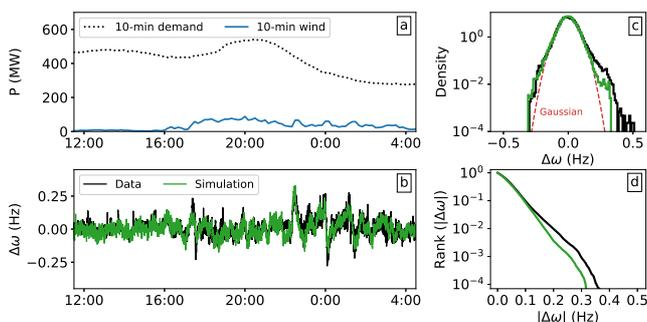
Fig. 1. (a) Evolution of demand and wind generation data [3]. (b) Time series, (c) probability density, and (d) rank size distribution of frequency fluctuations given by the model in comparison to the data [4].
