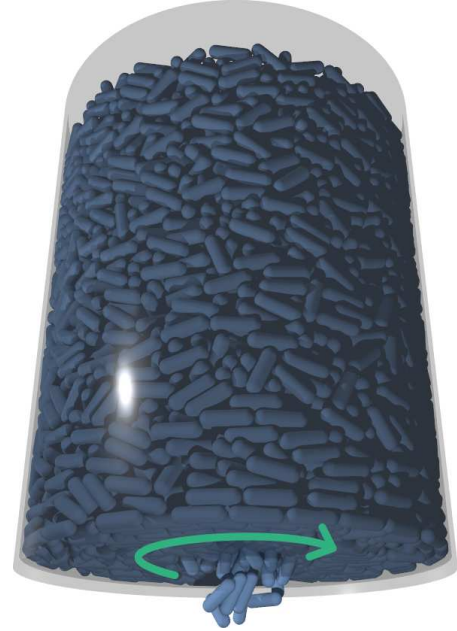
Fig. 1. Visualization of the numerical setup of the flat bottom, cylindrical silo with rotating bottom. Elongated particles are mimicked by spherocylinders.
