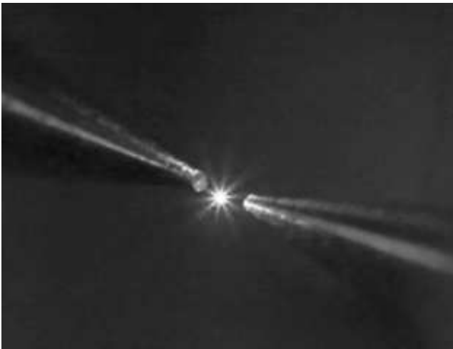
Fig. 1. Picture of a single nanodiamond (size = 100 nm) levitated by a Paul trap. The distance between the conical electrodes is 1.5 mm. The bright spot is due to the scattering of a laser beam focused at the position of the nanoparticle.
